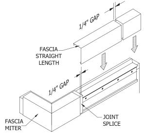
STEP 6b: Installing Fascia Radius Lengths Place a concealed joint splice in the opposite end of any adjacent piece. Install the fascia by hooking the top and pressing the top face downward to snap fascia into place. <u>Allow a</u> <u>1/4" gap between fascia sections for</u> <u>thermal expansion</u>. Review lengths of all pieces prior to cutting to avoid creating relatively short sections of fascia adjacent to full length sections.
